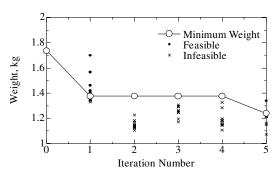
Fig. 5 Iteration history of the minimum weight for the MOGA.
