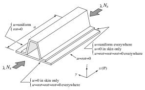
Fig. 1 Target hat-stiffened composite panel for structural optimization.
