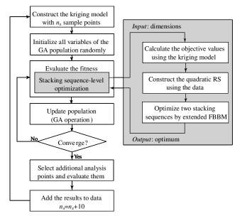
Fig. 3 Flowchart of multi-objective dimensions and stacking sequence optimization.
