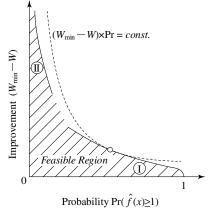
Fig. 2 Schematic representation of the Pareto frontier and curve of the normal EI method.
